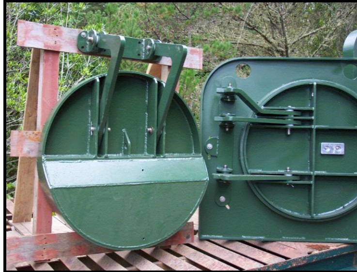
Figure 4-1. Top hinge (left) with internal float gate, and a side hinge (right) gate.
